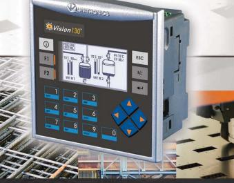
In these models certain inputs are adaptable, and can function as either digital, analog, and in certain models also as thermocouple or PT100. Using adaptable inputs reduces the amount of free digital inputs. For example, V130-33-RA22 offers 12 digital inputs. Implementing 2 TC inputs requires 4 digital inputs, leaving 8 free.
